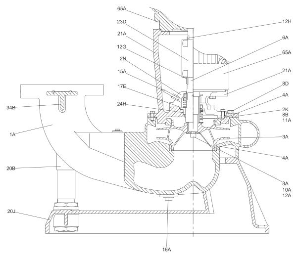
Fig. 2 VSM/VSMS cross-section
