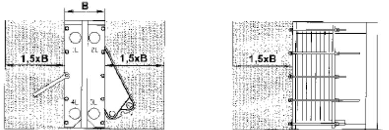
The values for the necessary space given in the adjacent figure are guide values and are recommended by Grundfos. You provide an adequate access to the plate heat exchanger.
